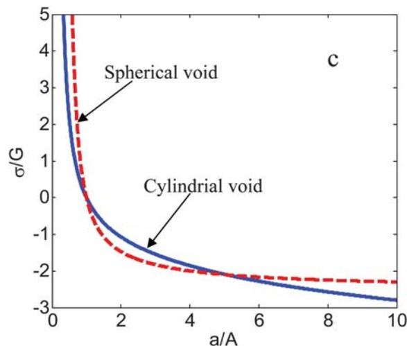
**Fig. 4** Under internal stress, the void changes size but retains shape, a mode of deformation which we call breathing. (a) Undeformed state. (b) Deformed state. (c) Normalized stress inside the void as a function of the normalized radius of the void ( $B/A \rightarrow \infty$ ).
