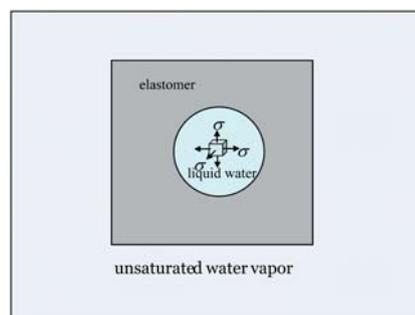
**Fig. 1** A void in an elastomer is filled with pure liquid water, and the elastomer is surrounded by unsaturated water vapor. The difference in humidity motivates water molecules to permeate through the elastomer, from inside the void to the outside of the elastomer. The osmosis leaves the liquid water inside the void in a state of triaxial tension.
