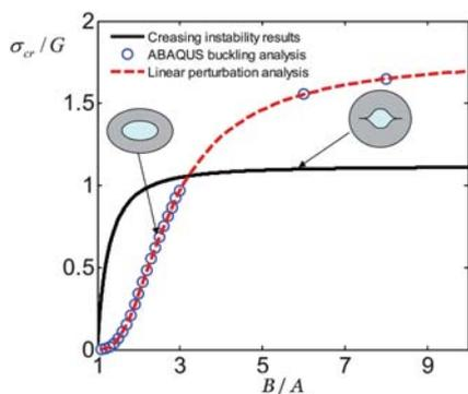
**Fig. 11** Buckling-to-creasing transition. The elastomer is a cylindrical shell, with inner radius  $A$  and outer radius  $B$  in the undeformed state. A thin shell buckles, and a thick shell creases.
