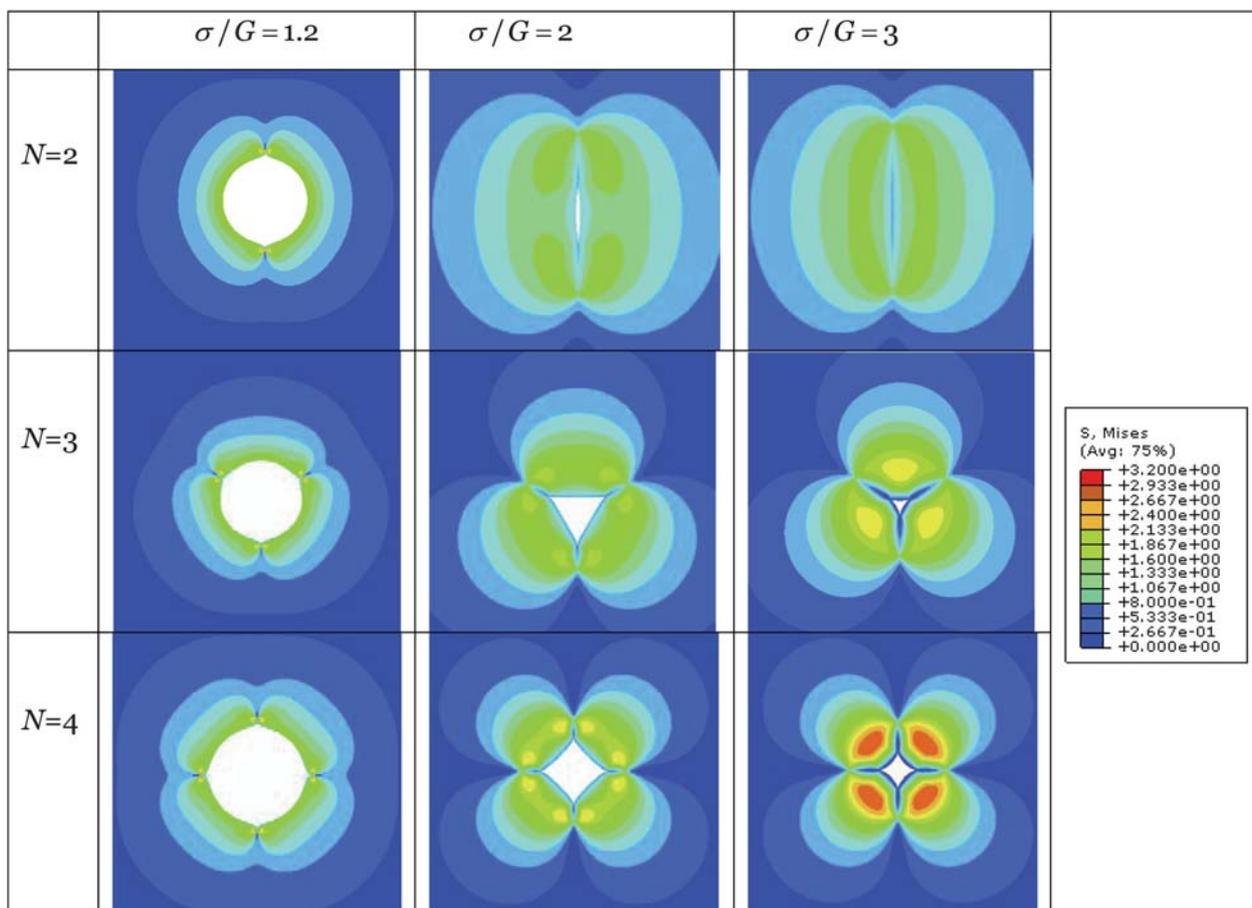
**Fig. 7** As the tension in the liquid water inside the void increases, the field of deformation in the elastomer evolves. The number of creases,  $N$ , is prescribed in the beginning of the simulation. The color indicates the level of the von Mises stress.
