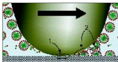
The AFM tip (moving left to right) in contact with both the substrate (1) and the micellar aggregates (2). Reprinted with permission from ref. 1. Copyright (2006) American Chemical Society.
