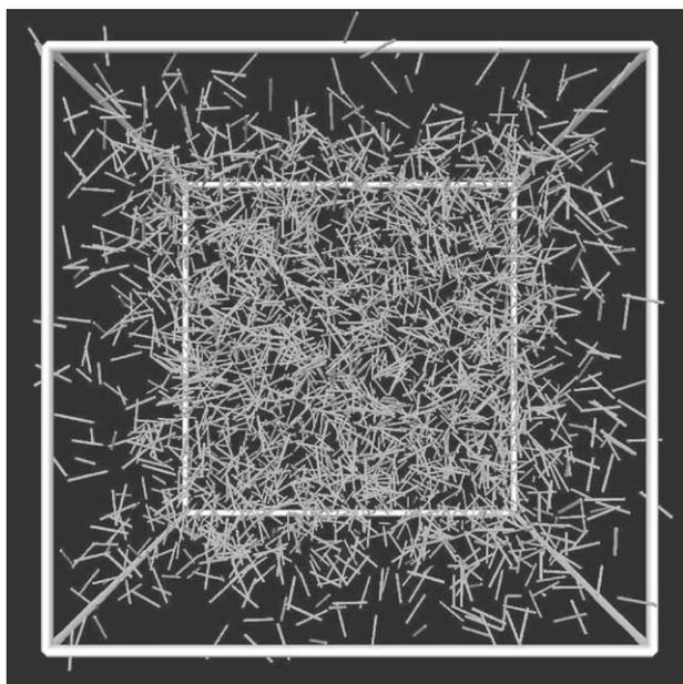
Fig. 9. Numerical simulation of percolation ( $\phi_c = 0.74\%$ ).
