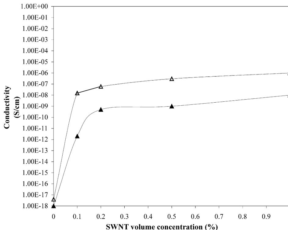
Fig. 4. DC surface and volume conductivity as a function of SWNT volume concentration [open triangle: volume conductivity (S/cm); closed triangle: surface conductivity (S)].
