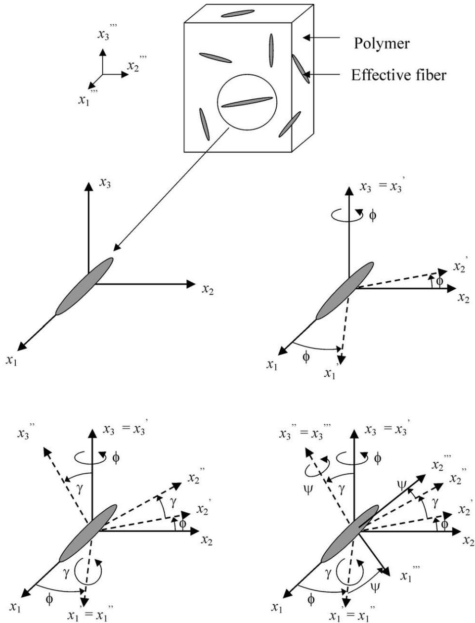
Fig. 4. Effective-fiber orientation.
