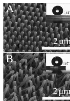
**Figure 4.** FE-SEM micrographs of PFPE-SS nanopillar films peeled from p-AAO membranes anodized at 180 V for (A) 10 min and (B) 15 min and pore-enlarged in 5% phosphoric acid aqueous solution at  $30^\circ\text{C}$  for 40 min. The inset in the top right corner of each image is the water droplet on the as-prepared PFPE-SS nanopillar film.
