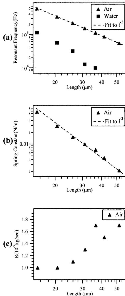
FIG. 3. (a) Measured resonant frequencies in air and water plotted as a function of length for an array of rectangular cantilevers which are 5  $\mu\text{m}$  wide and 86 nm thick. The resonant frequencies in air are fit to the expected  $(\text{length})^{-2}$  dependence. (b) Measured spring constants for the same cantilevers are plotted along with the fit, which predicts a  $(\text{length})^{-3}$  dependence. (c) The coefficients of viscous damping  $R$  as measured in air.
