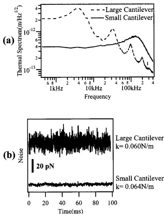
FIG. 4. (a) Thermal spectra of a large (200- $\mu\text{m}$ -long) and small (10- $\mu\text{m}$ -long) cantilever immersed in water far from the sample surface. (b) Measured force noise for the same two cantilevers in a 3 kHz bandwidth.
