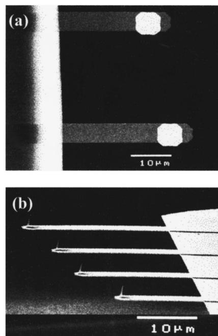
FIG. 2. (a) A SEM micrograph showing the top view of two small rectangular cantilevers with integrated reflector pads. The cantilevers are 5  $\mu\text{m}$  wide, 86 nm thick, and 27 and 32  $\mu\text{m}$  long. The pads are nominally 100 nm thick. (b) A SEM micrograph showing a perspective view of an array of cantilevers without pads. The tips were grown by electron beam deposition. The cantilevers are 5  $\mu\text{m}$  wide, 102 nm thick, and 14–24  $\mu\text{m}$  long.
