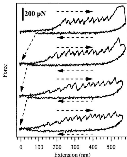
FIG. 5. (a) Four consecutive force spectra on a single molecule of the protein titin using a small cantilever. All force spectra were acquired at a pulling rate of 30–39  $\mu\text{m/s}$ , which is an order of magnitude faster than previously performed with conventional cantilevers.
