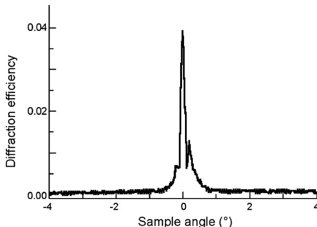
**Figure 6.** Typical Bragg peak obtained from photomonomer-filled L<sub>3</sub> silica. The diffraction strength exhibited does not reflect the maximum refractive index contrast available from the material and could be improved with optimized recording conditions.
