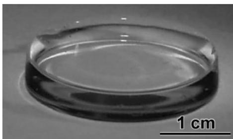
**Figure 2.** Representative silica sample following supercritical ethanol extraction. The original gel was cast into the shape of a disk using a Petri dish. The rim at the edge of the disk formed through the wetting of the dish by the liquid silica solution before gelling.
