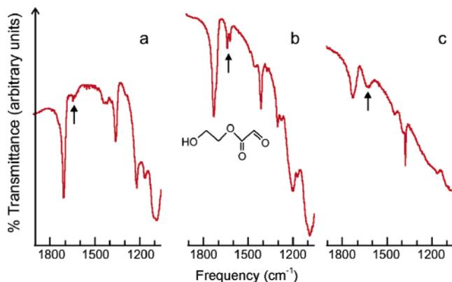
**Figure 5.** Infrared spectra of (a) porous silica before infiltration, (b) silica infiltrated with monomers of hydroxyethyl acrylate, and (c) silica after polymerization. The doublet peak indicated by the arrow in b is attributable to the monomer only and is diminished after polymerization (c).
