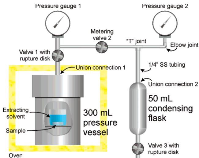
**Figure 1.** Schematic diagram of supercritical drying apparatus. The 300 mL pressure vessel was loaded with sample under ethanol and placed into a high-temperature oven (shaded square). The rest of the equipment was kept out of the oven.
