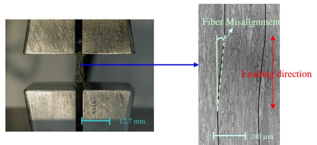
Figure 4. Compressive failure and fiber misalignment.
