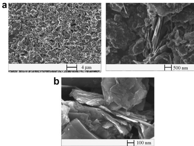
**Figure 1.** SEM images of graphite nanoplatelets: (a) before sonication; (b) after sonication.
