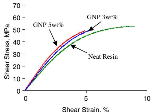
**Figure 2.** Shear stress–strain curve of nanocomposite with various nanoparticle loadings.
