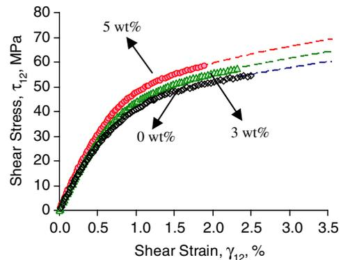
Figure 5. In-plane shear stress–strain curves for different nanoparticle contents (dashed lines extended from the experimentally obtained curves using  $\tau_{12} = k(\gamma_{12})^n$ ).
