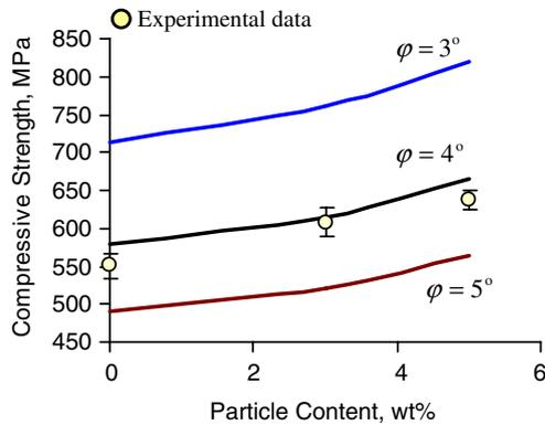
**Figure 6.** Comparison of measured and predicted compressive strengths for three values of fiber misalignment.
