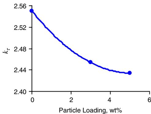
Figure 3. Shear stress concentration factor in fiber-reinforced composite.
