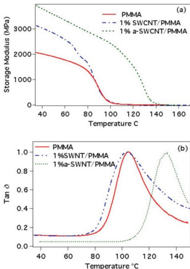
**Figure 5.** DMA results of the average of five test samples. (a) storage modulus and (b)  $\tan \delta$  with temperature sweep. [Color figure can be viewed in the online issue, which is available at [www.interscience.wiley.com](http://www.interscience.wiley.com).]
