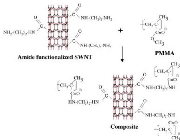
**Figure 1.** Proposed reaction scheme of amide-functionalized SWNT and PMMA composite. [Color figure can be viewed in the online issue, which is available at [www.interscience.wiley.com](http://www.interscience.wiley.com).]
