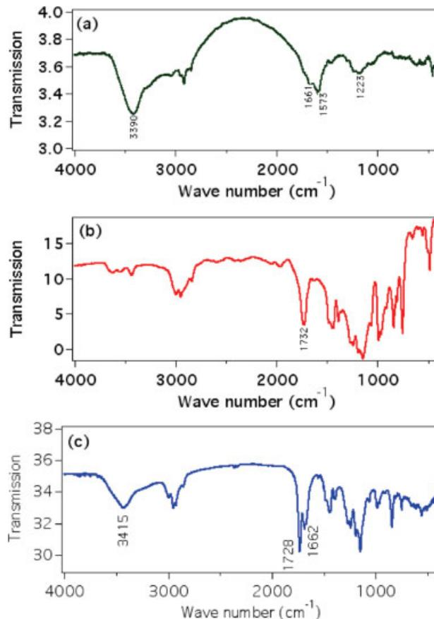
**Figure 2.** FTIR spectrum of (a) a-SWNT only, (b) PMMA only, and (c) a-SWNT-PMMA composites. [Color figure can be viewed in the online issue, which is available at [www.interscience.wiley.com](http://www.interscience.wiley.com).]
