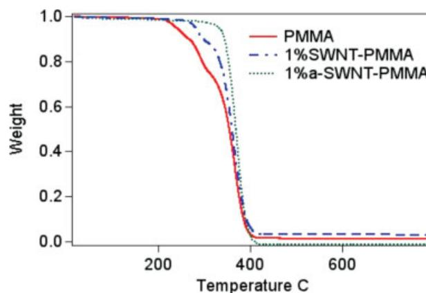
**Figure 4.** Thermogravimetric analysis of PMMA and its composites. Around 7 mg initial weight was used for this study, and normalized values are given for a comparison. [Color figure can be viewed in the online issue, which is available at [www.interscience.wiley.com](http://www.interscience.wiley.com).]
