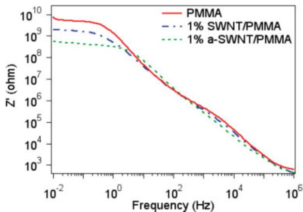
**Figure 8.** AC electrical impedance of nanocomposite, with frequency sweep at RT. [Color figure can be viewed in the online issue, which is available at [www.interscience.wiley.com](http://www.interscience.wiley.com).]
