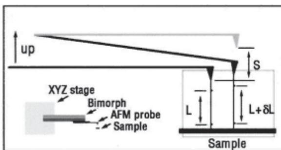
**Fig. 6.** Schematic showing the principle of the tensile-loading experiment. The cantilever is driven upward and it bends downward by a tip displacement  $S$ , while the nanotube is stretched from its initial length of  $L$  to  $L + \delta L$  because of the force exerted on it by the AFM tips. The force is calculated as  $k\delta L$ , where  $k$  is the force constant of the cantilever. The strain of the nanotube is  $\delta L/L$ .
