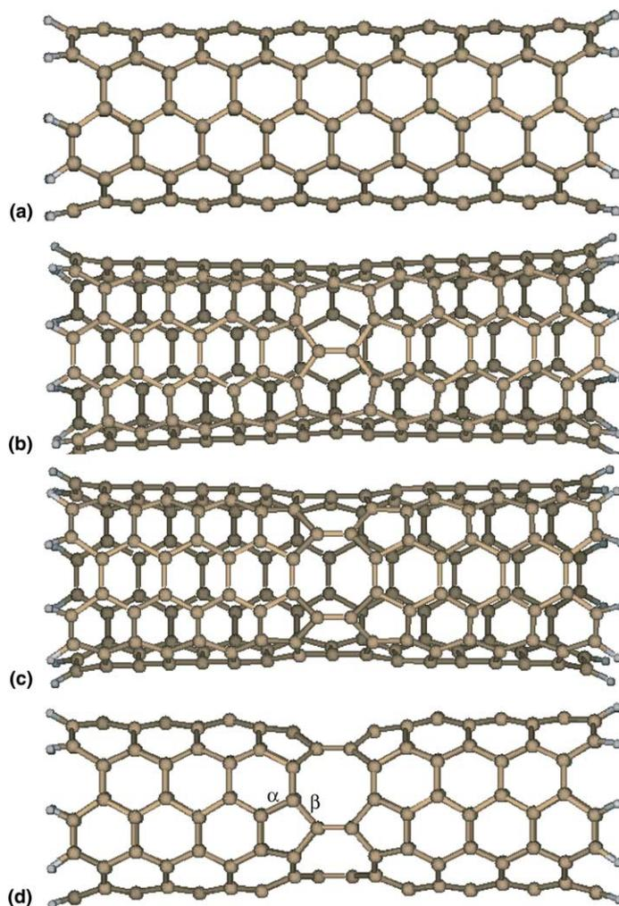
Fig. 1. Equilibrium structures of the [5,5] nanotubes included in this study: (a) pristine (defect free), (b) 1 defect, (c) 2 adjacent defects, (d) 5 adjacent defects.  $\alpha$  and  $\beta$  denote the two types of C–C bonds axially aligned within the pentagons.
