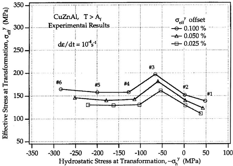
Fig. 9. Effective stress at the onset of transformation vs. the hydrostatic stress at the onset of transformation for a polycrystalline CuZnAl SMA specimen above  $A_f$ . Each number corresponds to a 1D or 3D loading (after Gall et al., 1998).
