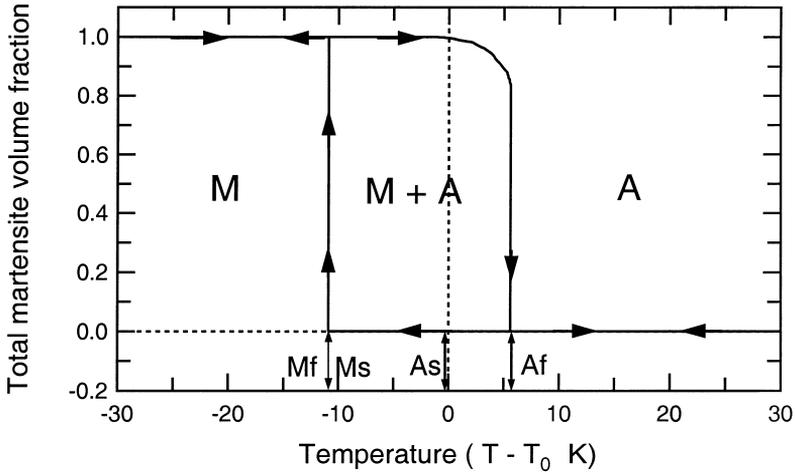
Fig. 2. Total martensite volume fraction vs. temperature for a temperature induced martensite transformation predicted by a 10-grain polycrystalline SMA.
