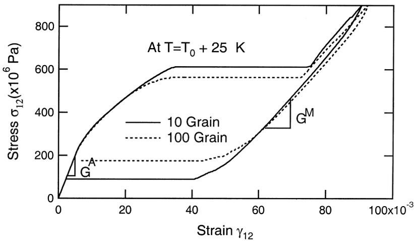
Fig. 3. Pseudoelasticity stress–strain curve for a 10-grain and a 100-grain polycrystalline specimen ( $T = T_0 + 25^\circ\text{K}$ ).
