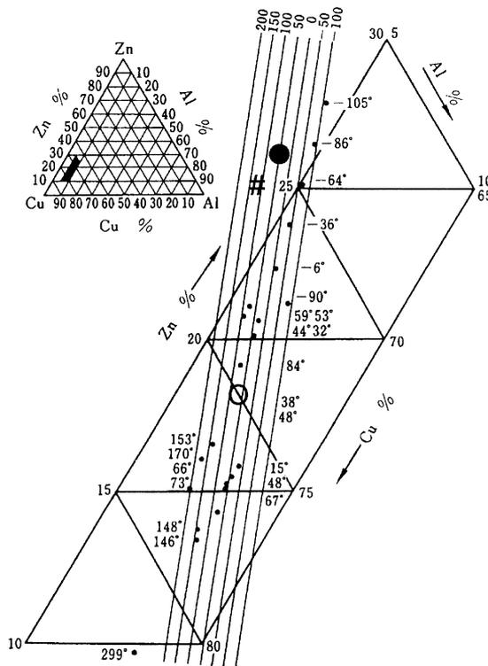
Fig. 12. A typical composition range for CuZnAl SMAs (after Delaey et al., 1978) showing the composition difference between the experimental specimen and model specimen (#, experimental,  $\text{Cu}_{71}\text{Zn}_{25}\text{Al}_4$  wt.%; ●, model,  $\text{Cu}_{70}\text{Zn}_{26}\text{Al}_4$  wt.%; ○, model,  $\text{Cu}_{75}\text{Zn}_{17}\text{Al}_8$  wt.%).
