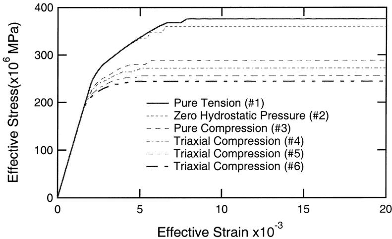
Fig. 10. Model predicted effective stress–strain plots for a polycrystalline CuZnAl SMA specimen at about  $(M_s + A_s)/2$ . Each one of the curves corresponds to a 1D or 3D loading.
