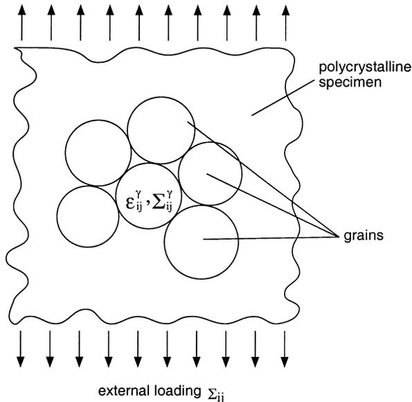
Fig. 1. Polycrystalline specimen is modeled as a number of random-oriented, spherical, single-crystalline grains.
