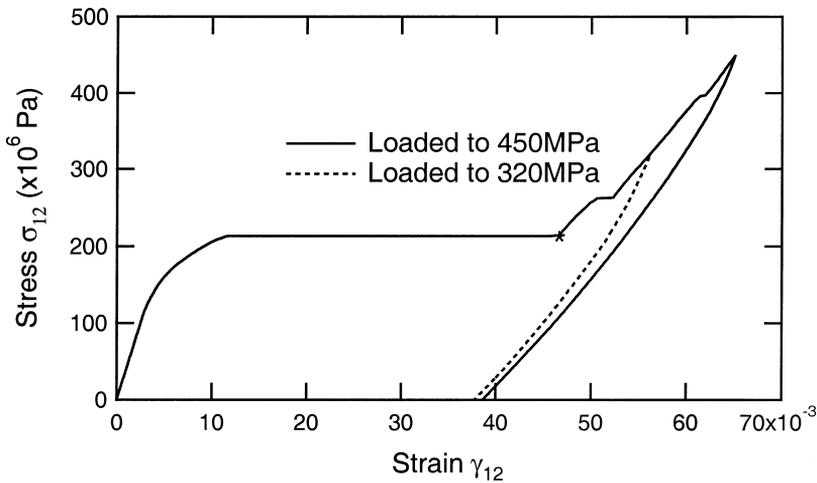
Fig. 5. Stress–strain curve of a 10-grain polycrystalline specimen at temperature  $T = T_0$  predicted by the model. \*, forward transformation to 100% martensite.
