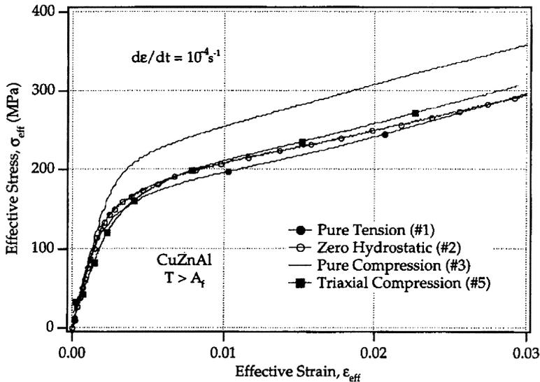
Fig. 8. Effective stress–strain plots for a polycrystalline CuZnAl SMA specimen above  $A_f$ . Each one of the curves corresponds to a 1D or 3D loading (after Gall et al., 1998).
