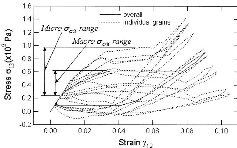
Fig. 4. Stress–strain curve of overall specimen and individual grains for PE of 10-grain specimen.
