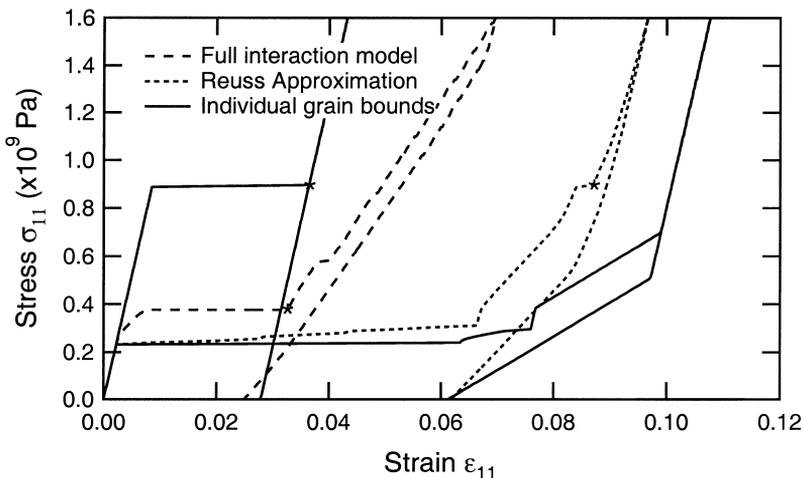
Fig. 7. Stress–strain curves predicted by both Reuss approximation and polycrystal model for a 10-grain polycrystalline specimen. Forward transformation to 100% martensite is indicated by \* on each curve.
