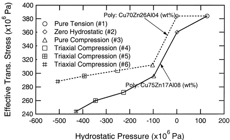
Fig. 11. Model predicted effective stress at 100% transformation vs. the hydrostatic stress at 100% transformation for a polycrystalline CuZnAl SMA specimen at about  $(M_s + A_s)/2$ . Each number corresponds to a 1D or 3D loading.
