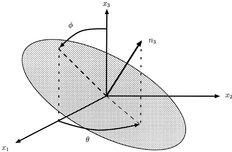
Fig. 5. The orientation of a penny-shaped martensite plate relative to austenite material axes  $x_1$ ,  $x_2$ , and  $x_3$ . Normal,  $n_3$ , is parallel to smallest dimension of penny ( $a_1 = a_2 > a_3$ ).
