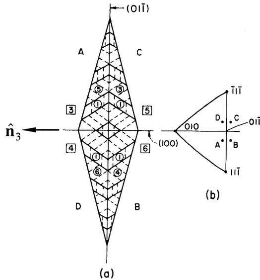
Fig. 2. (a) Geometry of  $(01\bar{1})$  plate group for 2H martensite. Solid line: twin boundaries and boundaries between variants. Dashed line: basal planes. (b) Habit plane normals of the variants in (a) in a  $(01\bar{1})$  standard projection (after Saburi and Wayman, 1979).
