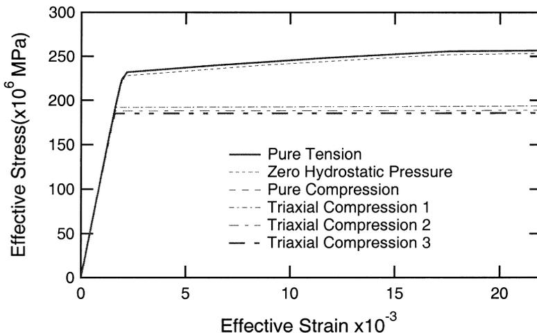
Fig. 11. Model predicted effective stress–strain curves for a CuZnAl single crystal under different uniaxial and triaxial loading states (see Part 2 for description).
