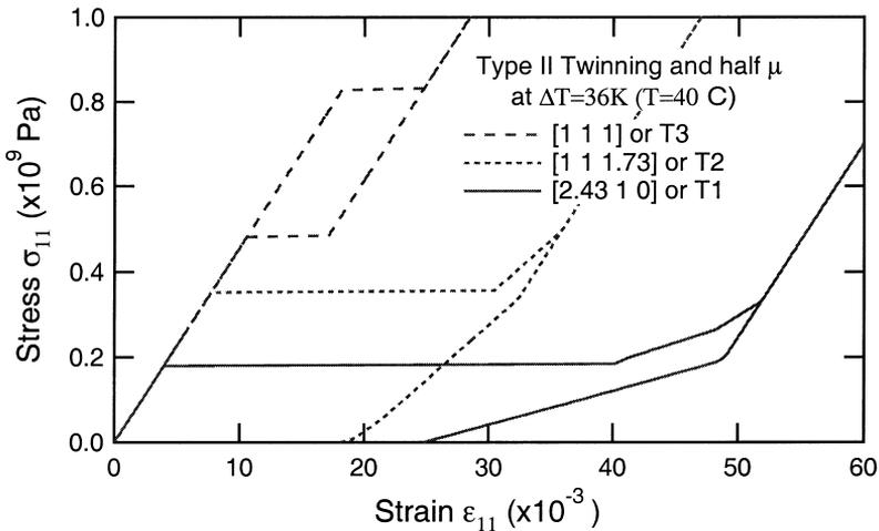
Fig. 10. Model predicted results for a Cu–14.2Al–4.3Ni (wt.%) alloy under different uniaxial loading directions. The temperature is set to be  $\Delta T = 36\text{K}$ , type II twinning is used as the lattice invariant shear and the shear modulus is reduced by half.
