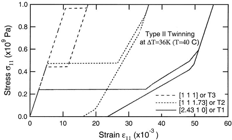
Fig. 8. Model predicted results for a Cu–14.2Al–4.3Ni (wt.%) alloy under different uniaxial loading directions. The temperature is set to be  $\Delta T = 36\text{K}$  and type II twinning is used as the lattice invariant shear.
