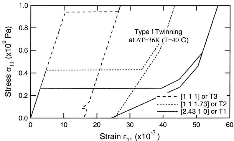
Fig. 9. Model predicted results for a Cu–14.2Al–4.3Ni (wt.%) alloy under different uniaxial loading directions. The temperature is set to be  $\Delta T = 36\text{K}$  and type I twinning is used as the lattice invariant shear.
