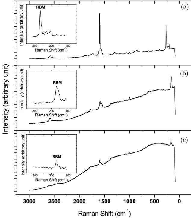
Fig. 2. Raman spectra of SWNT/polyimide nanocomposites: (a) 0.1 wt% HiPCO-SWNT, (b) 0.1 wt% P2-SWNT, and (c) 0.1 wt% P3-SWNT. A 785-nm (1.58 eV) incident laser light excitation with a 25- $\mu\text{m}$ -slit aperture was used.
