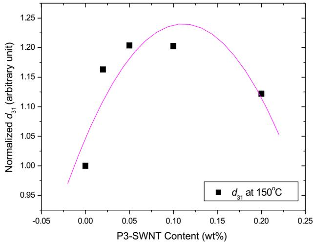
Fig. 9. Normalized piezoelectric strain coefficient ( $d_{31}$ ) of P3-SWNT/polyimide nanocomposites as a function of SWNT concentration.
