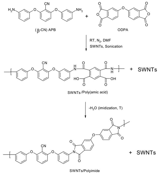
Fig. 1. Schematic diagram of synthesis of SWNT/polyimide nanocomposite.
