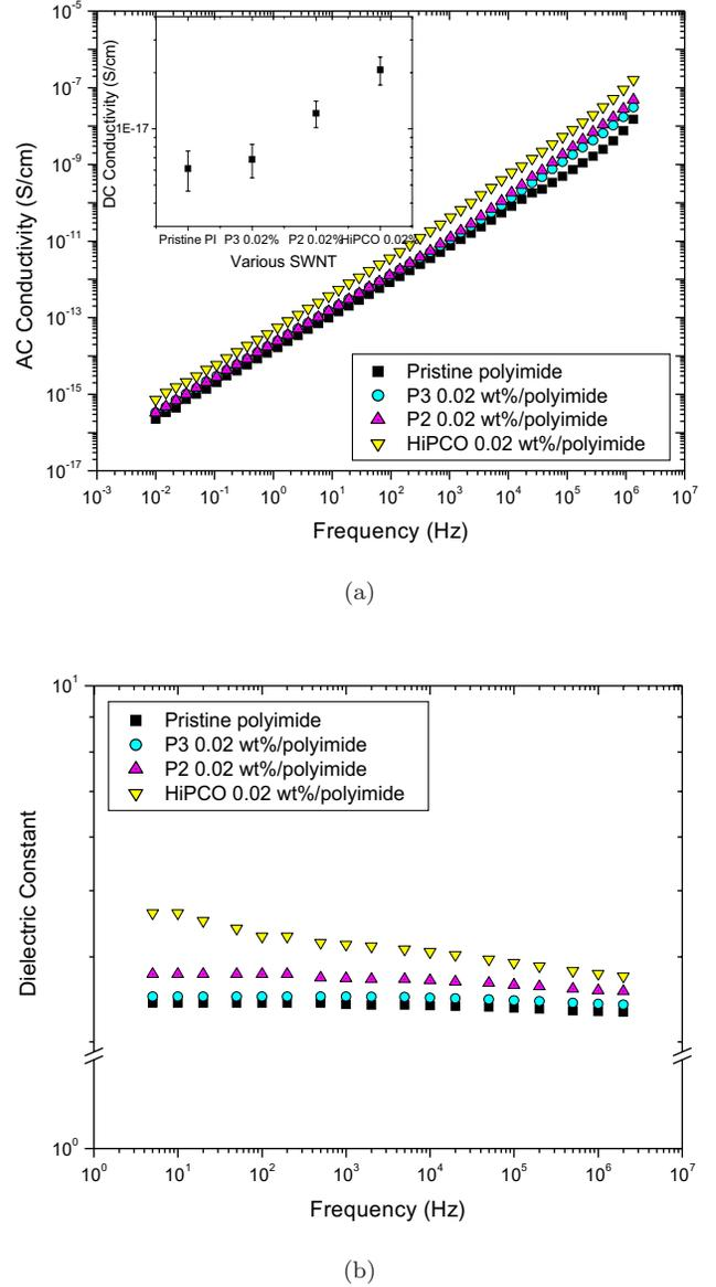
Fig. 4. (a) AC and DC electrical conductivity and (b) dielectric constant of 0.02 wt% SWNT/polyimide nanocomposites.
