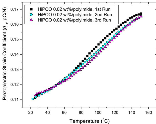
Fig. 10. Piezoelectric strain coefficient ( $d_{31}$ ) of 0.02 wt% HiPCO-SWNT/polyimide nanocomposites as a function of temperature for three cycles.
